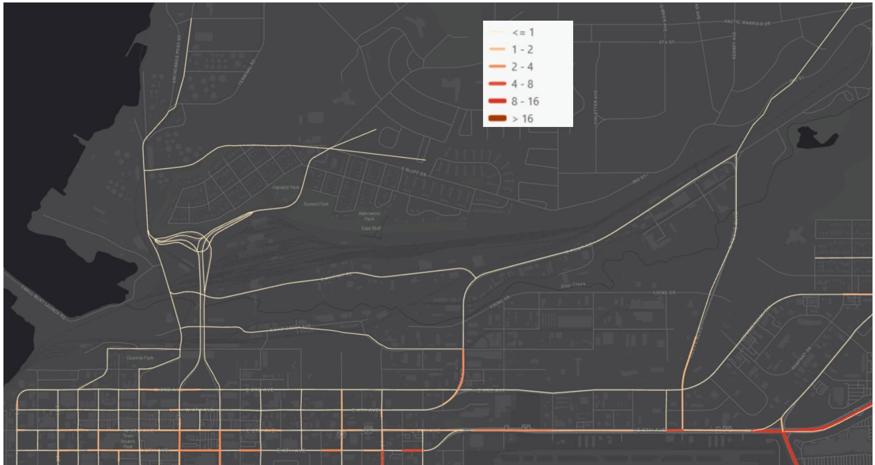
FIGURE 28: 2019 PM PEAK HOUR (5PM TO 6PM) VEHICLE HOURS OF DELAY (VHD) IN NORTH PART OF THE PROJECT AREA
