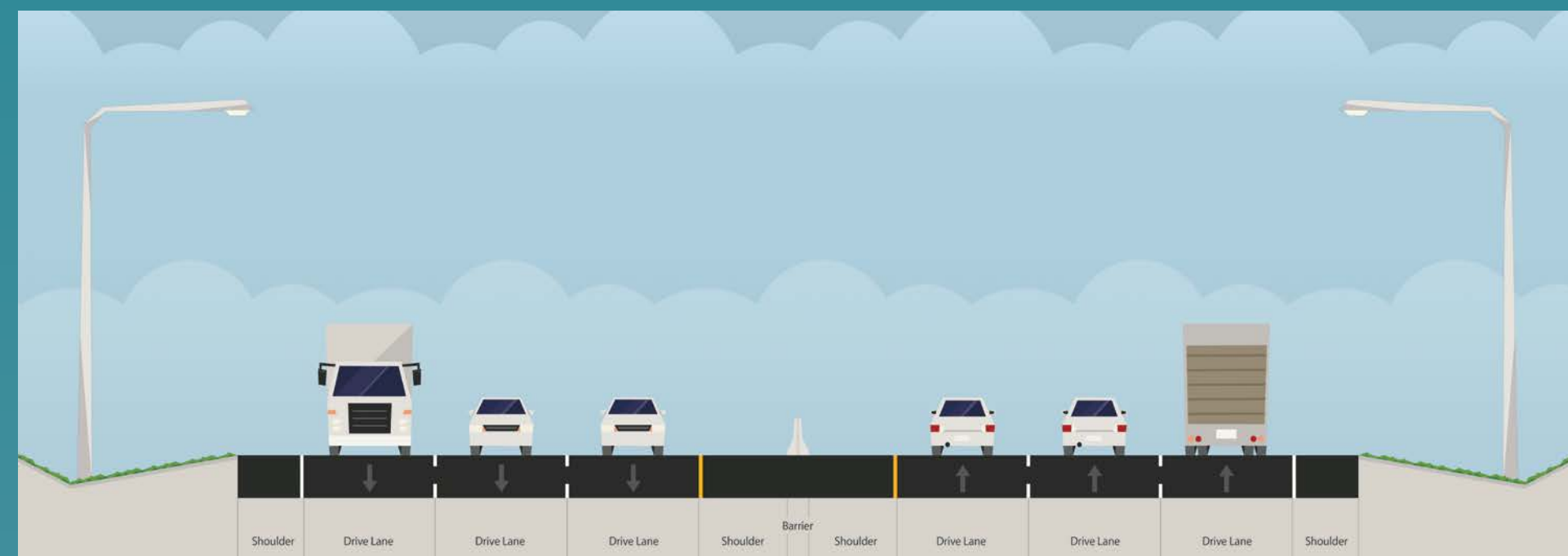
Concrete Barrier Median (Potential Future Build-Out)
