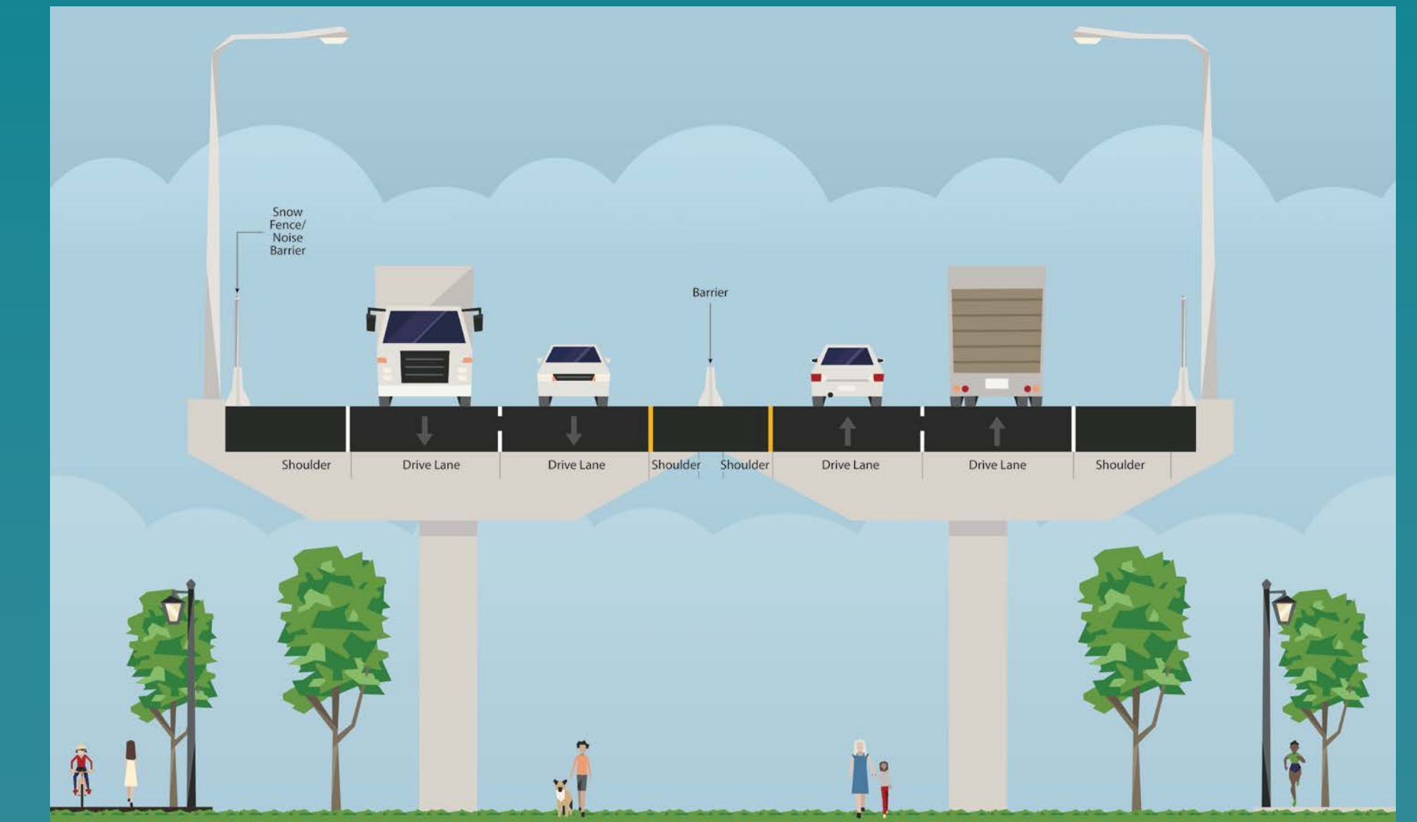
Elevated Section with 4 Lanes
