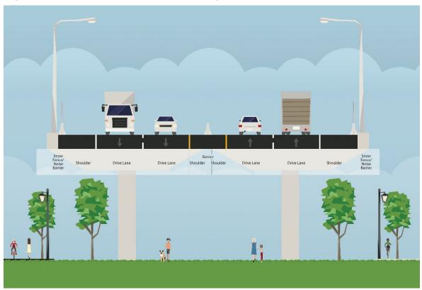
Figure 28. Cross-Section of Viaduct Bridge over a Park
