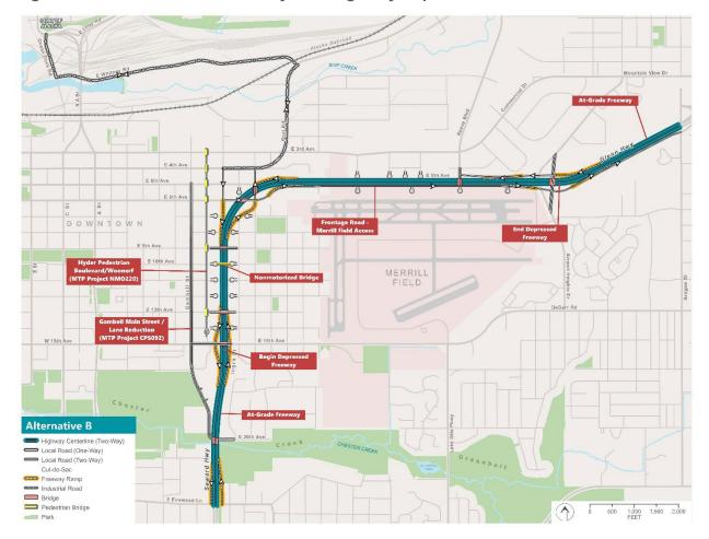
Figure 16. Alternative B: Roadway and Highway Improvements
