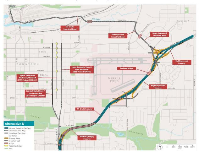
Figure 27. Alternative D Roadway and Highway Improvements
