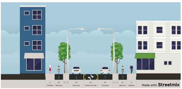
Figure 13 shows a concept for a potential Ingra Street that fits within the existing 60-foot-wide right-of-way. It features a shared directional cycle track/sidewalk (see Figure 14) on each side and includes a center turn lane to access driveways or side streets. A 4-foot buffer would separate the vehicle travel lanes from the nonmotorized facilities.
