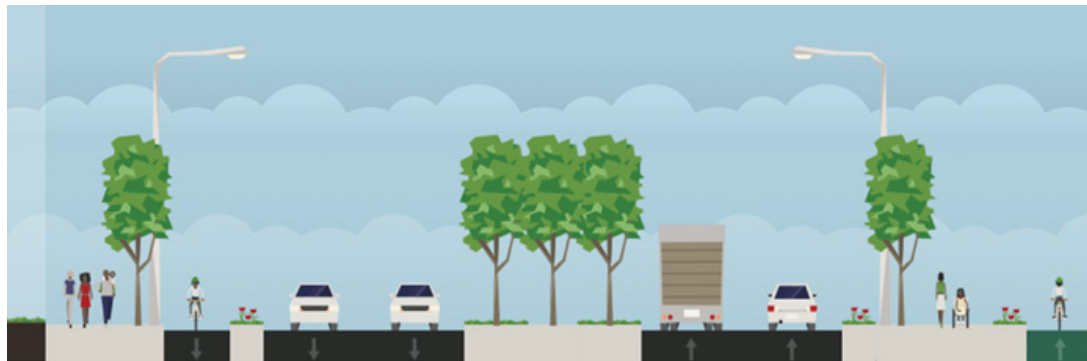
Figure 16: Potential parkway south and east of Merrill Field. This graphic shows one potential cross-section of the Fairview Bypass which is proposed as a parkway. Various non-motorized improvements and/or landscaping configurations are possible while still staying within the proposed 125-foot right-of-way south and east of Merrill Field.
