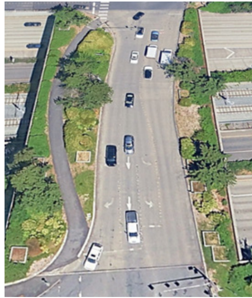
Figure 15: This image shows a bridge of Island Crest Way over I-90 in Seattle. It depicts the concept proposed for crossings of Karluk and Medfra Streets. The extra-wide bridges would allow for a separated trail and landscaping, and shield surface users from the traffic below.
